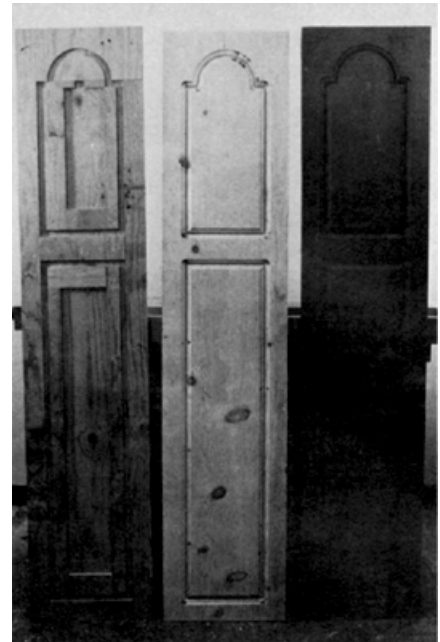
From left to right: A router arm template for a paneled shutter, the routed shutter board, and the finished shutter.
