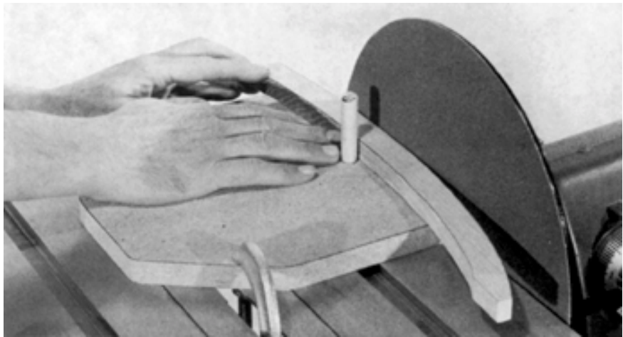
Figure 17-20. Use a guide to sand curved workpieces to a uniform width. The edge that bears against the dowel must be smooth and true.
