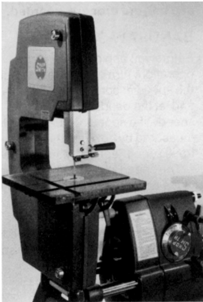
Figure 14-1. The Bandsaw can be mounted on (A) the Mark V or (B) on a Shopsmith Power Stand.
