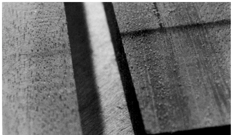
Figure 21-10. It's normal for the planer to cut a small snipe (less than 0.005" deep) in the end of a board as shown on the right. But if you let a board droop when it's fed into or coming out of the planer, the knives may cut a pronounced snipe in one end as shown on the left. Keep the board parallel to the flat on the table at all times.
