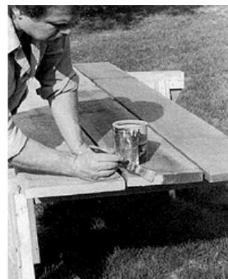
Figure 3. Paint the ends of the boards to prevent them from checking. If left unpainted, the ends will dry out faster than the rest of the board.
